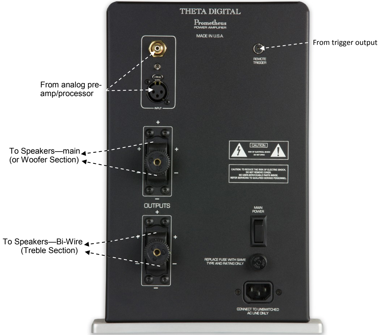
Figure 5 - Examples of Typical Input and Output Connections
